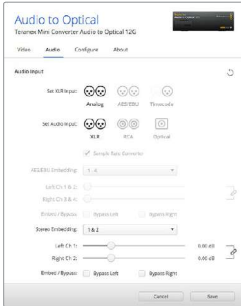
Adjust your analog audio levels and AES/EBU levels using the ‘audio’ settings page in Blackmagic Teranex Setup.
