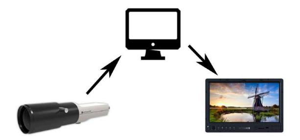
We recommend probes that can handle at least 2000 nits of brightness and 1:100000 contrast ratios (depending on your monitor Nit level, your probe should handle more). Common professional calibration probes include the <u>Klein Instruments K-10A</u> and Colorimetry Research CR-100. More budget probes are available on the market, you will get what you pay for in many cases.
