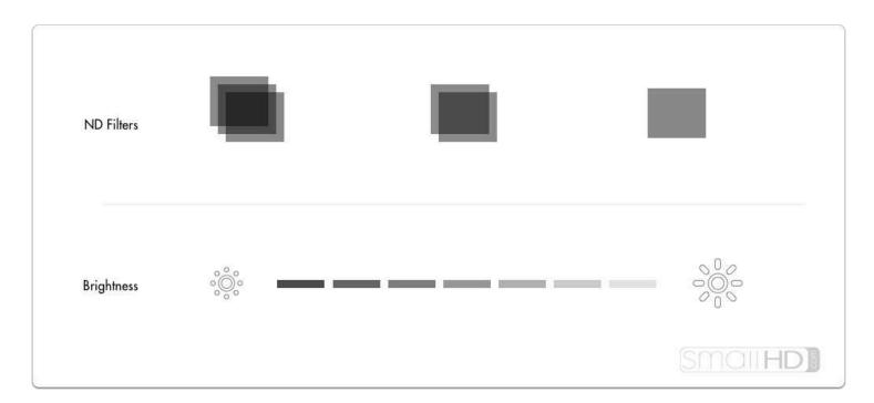
Lens filters offer creative flexibility on brightly lit scenes - instead of having to raise shutter speed and increase strobing, or close down the aperture and deepen the depth of field, ND (neutral density - aka darkening) filters can darken the shot without adjusting the aesthetic.
