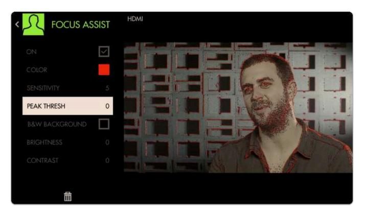
Bringing **Peak Threshold** up to around 30 does a better job of causing **only in-focus areas to activate the filter** but this is ultimately a balance that may need tweaking depending on the camera/shot.
