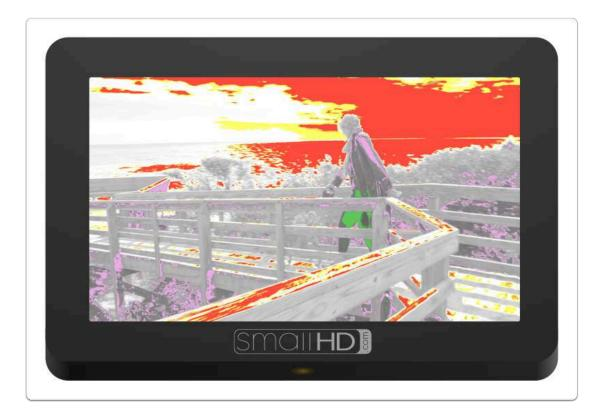
Exposure Assist is a great overall balance of utility and ease of use and can benefit most shooting scenarios. It allows 'painting' the image depending on the intensity of a pixel's luma value. For example you could set 97% IRE and up to turn bright red as an overexposure warning while creating a scale to turn green when a face is exposed properly at 55%, etc. (& anything else you wish to plot to any points on the range). <u>Click to learn more about Exposure Assist.</u>
