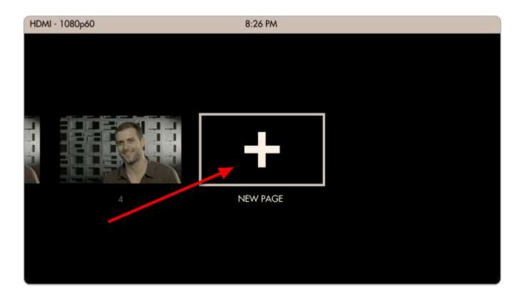
The entire monitor is based on the concept of customizablePages- instead of having to enable and disable features individually when needing to change a setup, create pages with a task in mind, for example setting exposure, and quickly joystick (switch) between each page on-set for a highly efficient workflow.
