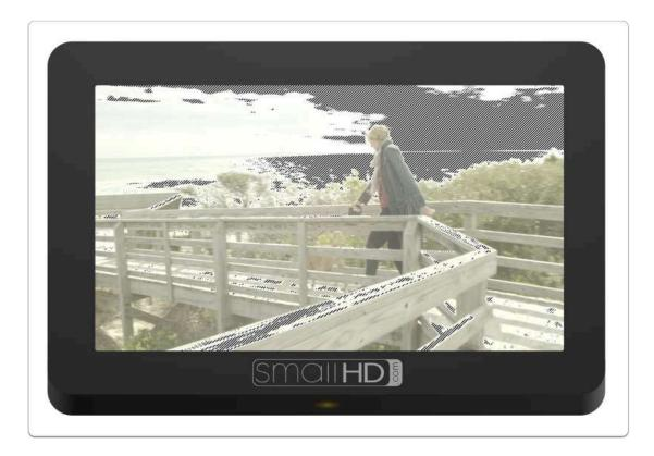
Zebra is essentially a simplified version of Exposure Assist which allows the specific 'painting' of areas depending on brightness value but is less destructive to the underlying image -- it is however limited to painting one value range at a time, though up to two Zebra tools can be activated simultaneously. <u>Click to learn more about the Zebra tool</u>.
