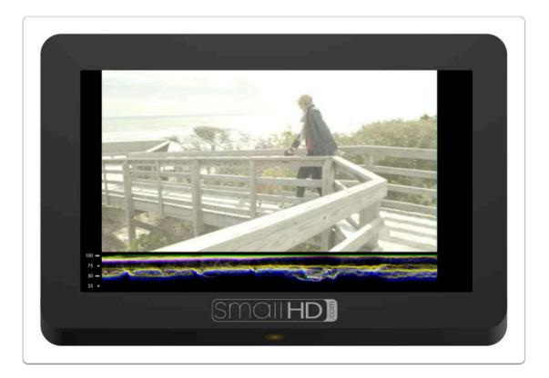
Waveform plots the value of the entire image onto a graph that physically matches it from left-to-right, meaning if you see an area that's too bright on the left side of the image, it will create a 'peak' on the left side of the waveform graph. It also has other benefits by way of RGB & RGB Parade modes. <u>Click to</u> <u>learn more about the Waveform.</u>
