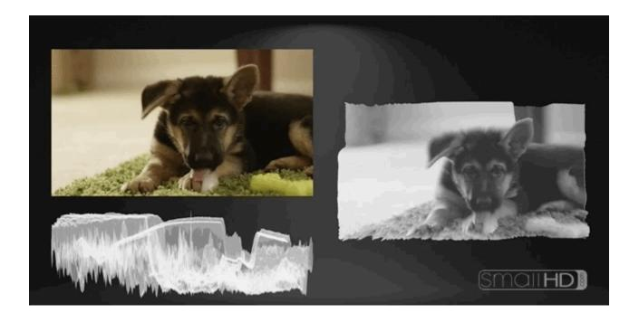
The Waveform is generally considered the most robust exposure tool because it plots your image's luminance (brightness) -- and chrominance if using RGB mode -- to a graph but unlike the Histogram, it physically matches the screen from left-to-right.
