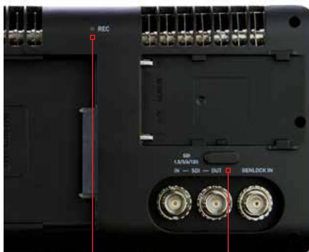
Tally Light Flashes red when recording
